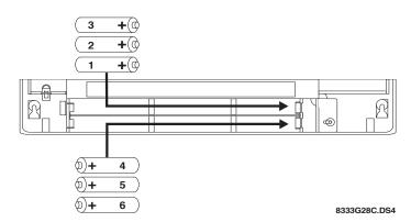
Figure 7. Battery Polarity and Order of Installation
