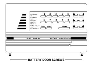
Figure 5. Loosen the two battery door screws
