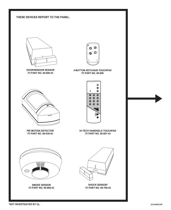
Figure 1. Typical System Components
