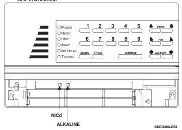
Figure 6. Tab Indicates Battery Type Installed
