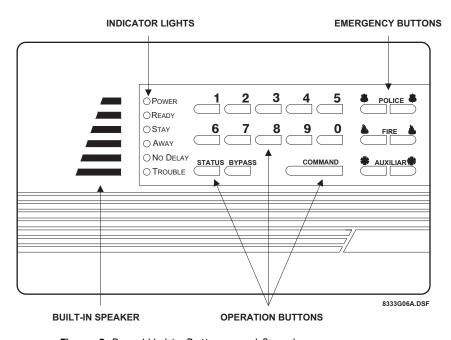
Figure 2. Panel Lights, Buttons, and Speaker
