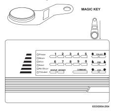
Figure 3. Inserting the Magic Key into the Slot
